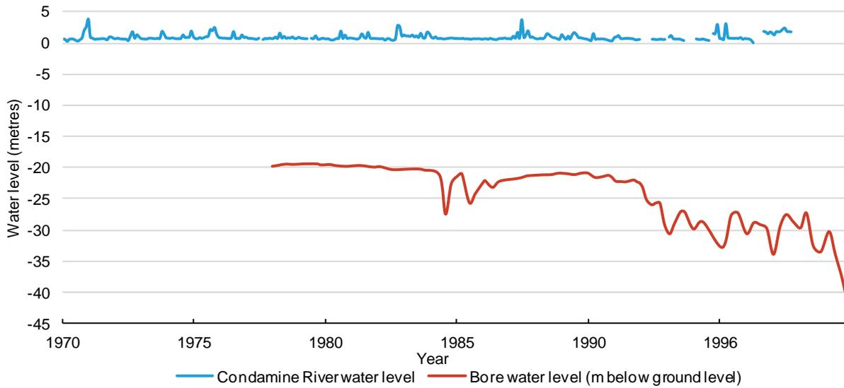
**Figure 32 Hydrograph from the gauging station at Loudouns Bridge (Central Condamine Alluvium) on the Condamine River and bore hydrograph from a monitoring bore approximately 13 km east of the river in the Condamine Alluvium (42231195)**
