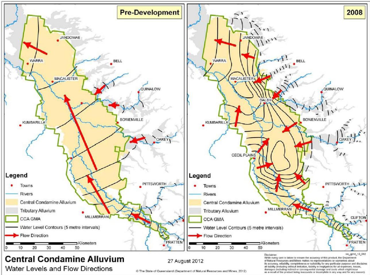
**Figure 24 Effect of groundwater developments on groundwater levels and flow directions**
