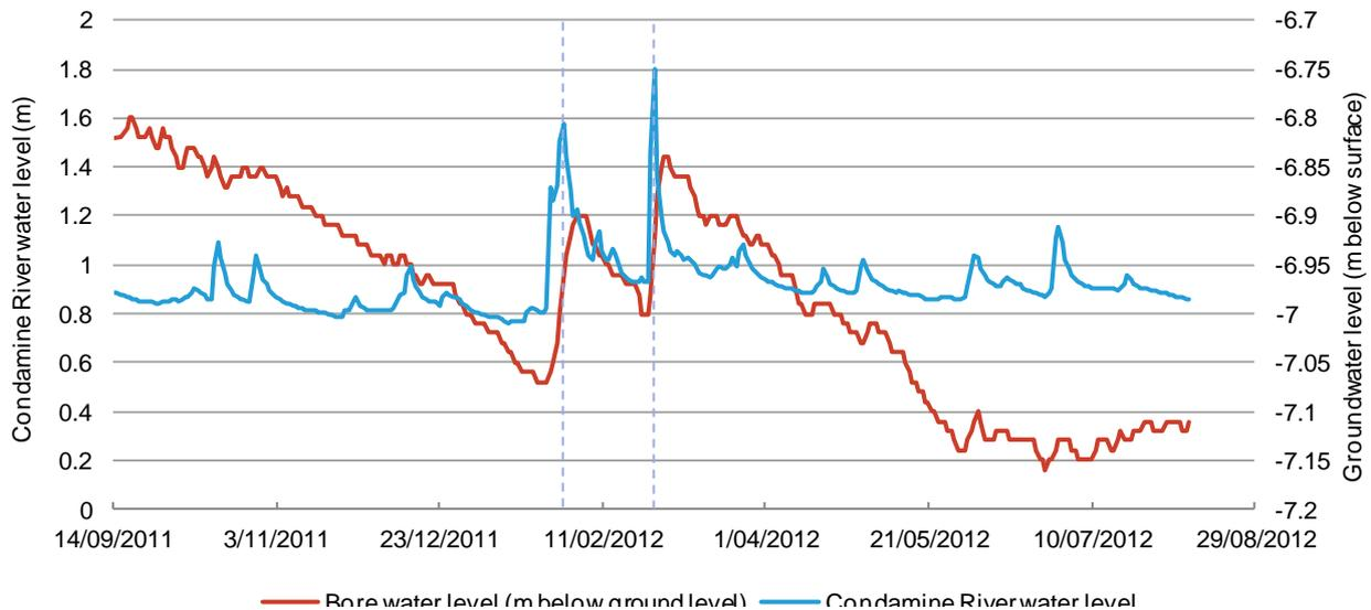
**Figure 33 Hydrograph from the gauging station at Warwick (upper reaches of Condamine Alluvium) on the Condamine River and bore hydrograph from a monitoring bore approximately 4 km away in the Condamine Alluvium (42231672)**
