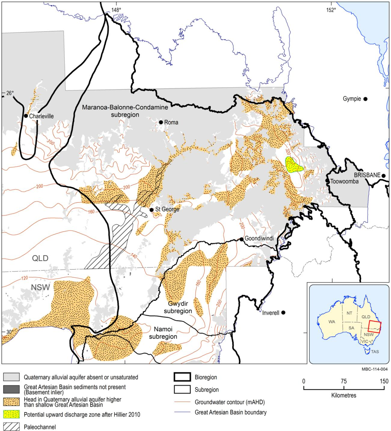
**Figure 23 Groundwater levels in the shallow alluvial system (Narrabri Formation) showing areas where groundwater heads are higher than in the upper parts of the Great Artesian Basin**
