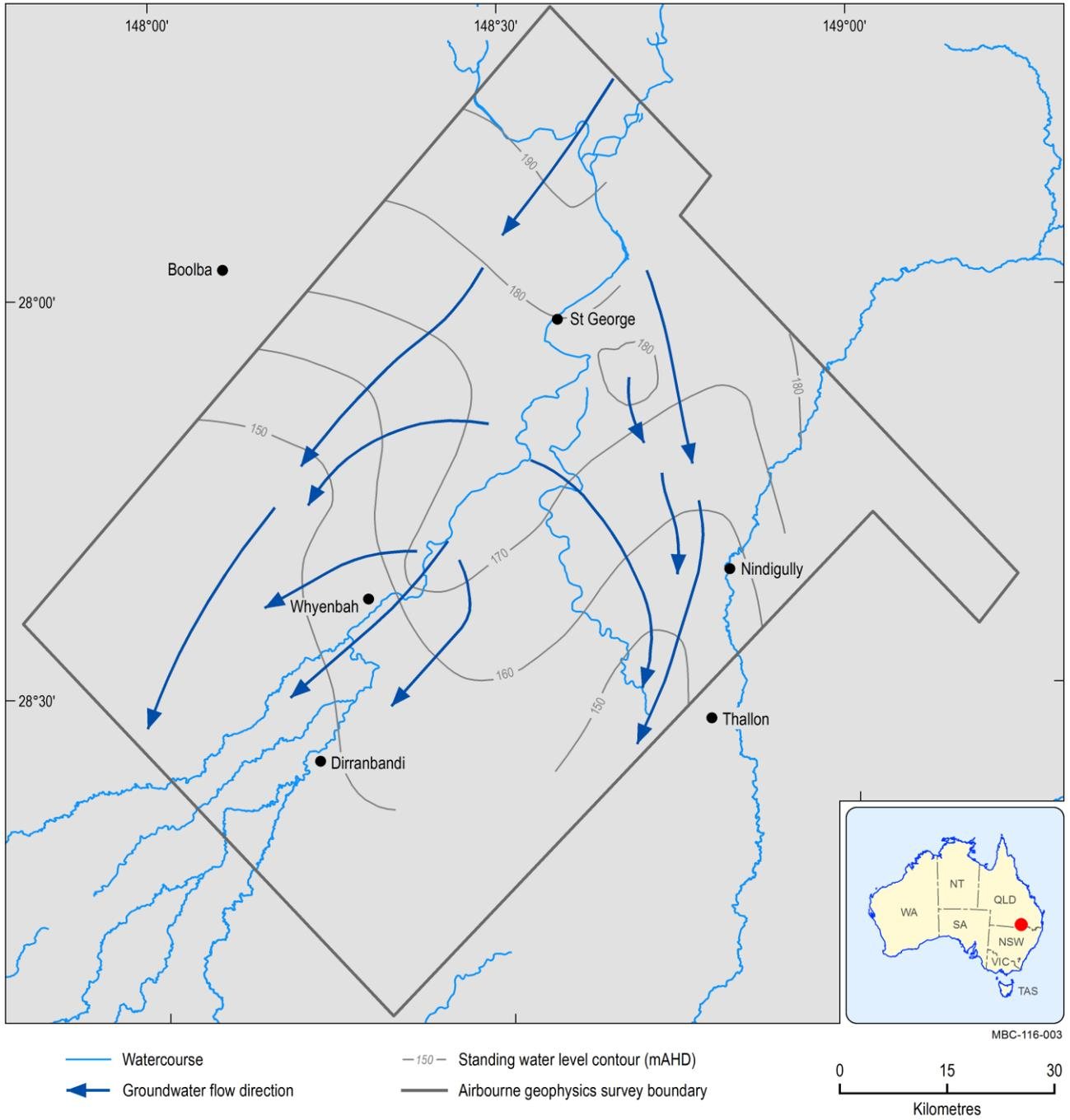
**Figure 34 Watertable contours and groundwater flow directions, upper alluvial aquifer**
