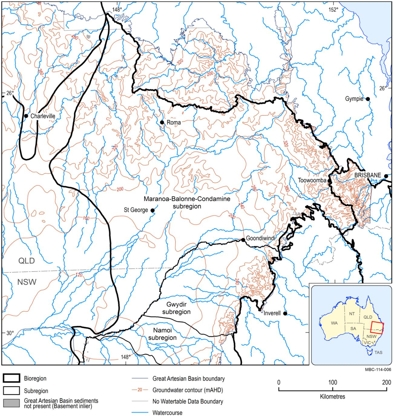
**Figure 25 Groundwater level contours for the upper units of the Surat Basin**
