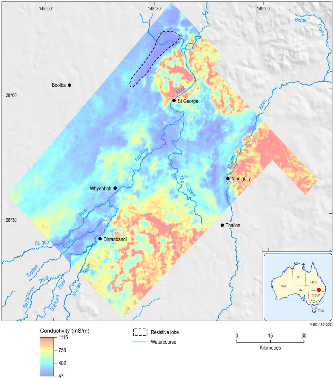
**Figure 35 Representative 30 to 40 m airborne electromagnetic conductivity slice, showing a resistive lobe in the north**
