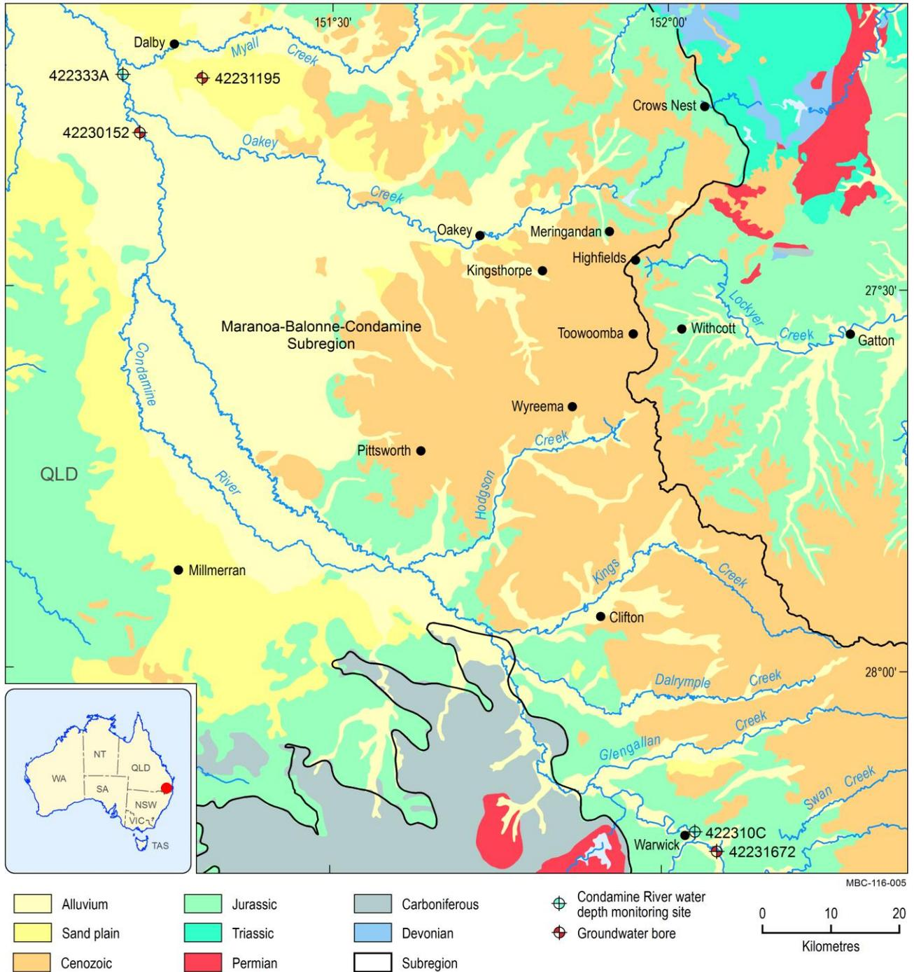
**Figure 30 Surface geology of the Condamine Alluvium area showing the location of selected river gauging stations and groundwater monitoring sites**
