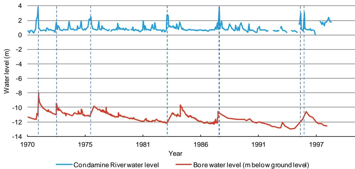
**Figure 31 Hydrograph from the gauging station at Loudouns Bridge (Central Condamine Alluvium) on the Condamine River and bore hydrograph from a monitoring bore approximately 9 km upstream (Registered Number 42230152)**
