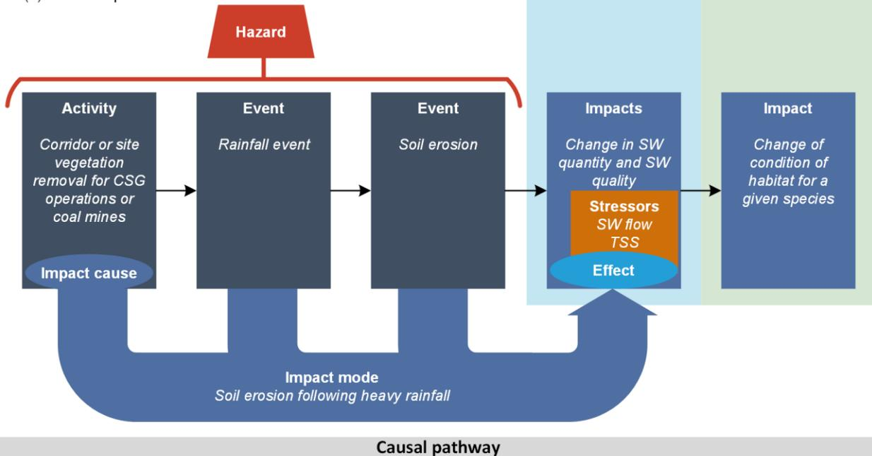
**Figure 6 Hazard analysis using the Impact Modes and Effects Analysis**
