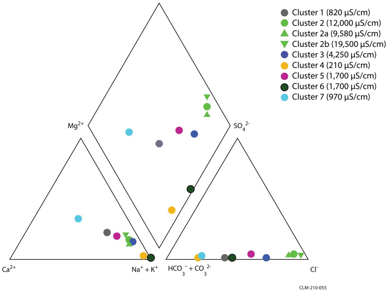
**Figure 55 Piper diagram showing the major ion relationships of different bedrock hydrochemical clusters in the Clarence-Moreton bioregion (based on the median concentrations shown in Table 15)**
