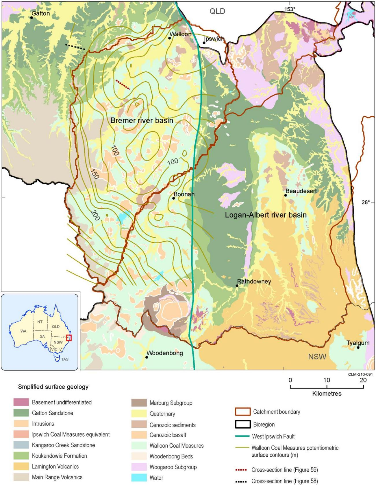
**Figure 69 Piezometric surface map of Walloon Coal Measures in the Bremer river basin**
