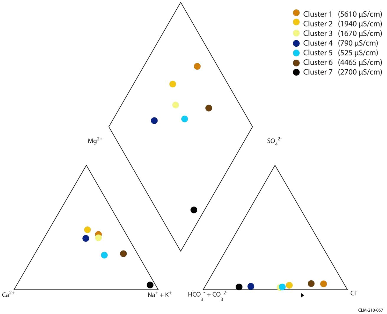
Figure 56 Piper diagram showing the major ion relationships of hydrochemical clusters in the Lockyer Valley (based on the median concentrations shown in Table 17)
