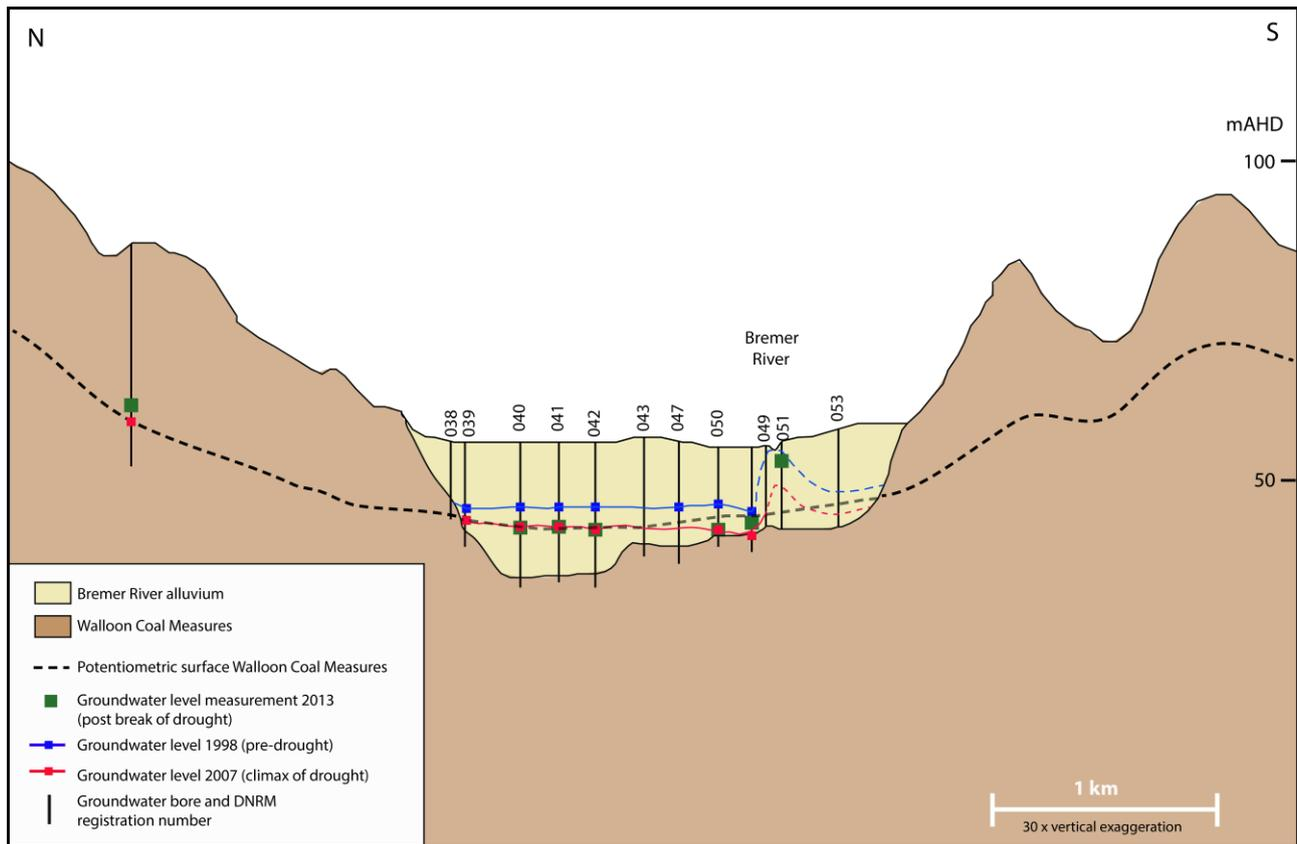
**Figure 67 Geological cross-section through the Bremer river basin**
