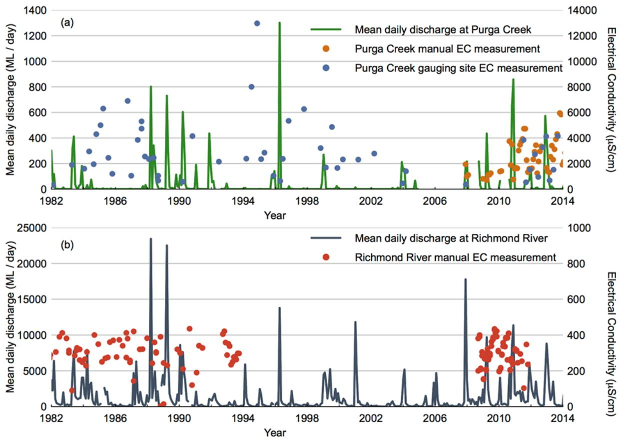
**Figure 65 Electrical conductivity (EC) measurements and mean daily discharge at (a) Purga Creek at Loamside in the Bremer river basin and (b) Richmond River at Casino**
