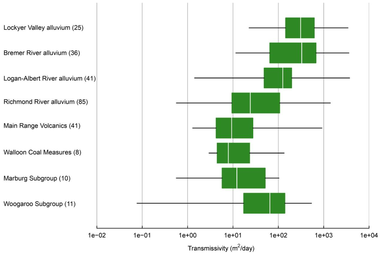
**Figure 52** Box plot to show the transmissivity range of aquifers with enough data
