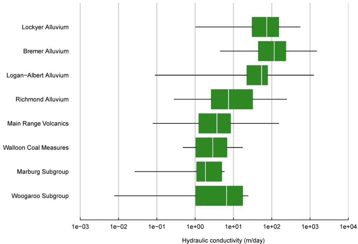
**Figure 53** Box plot to show the hydraulic conductivity range of aquifers with enough data
