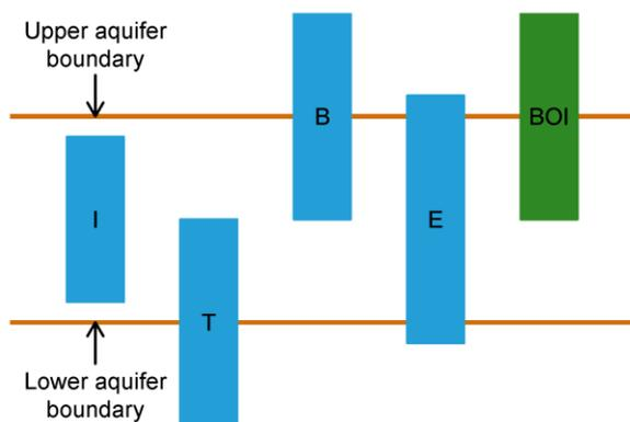
**Figure 19** Diagram showing the spatial relationship between aquifer boundaries and screen intervals
