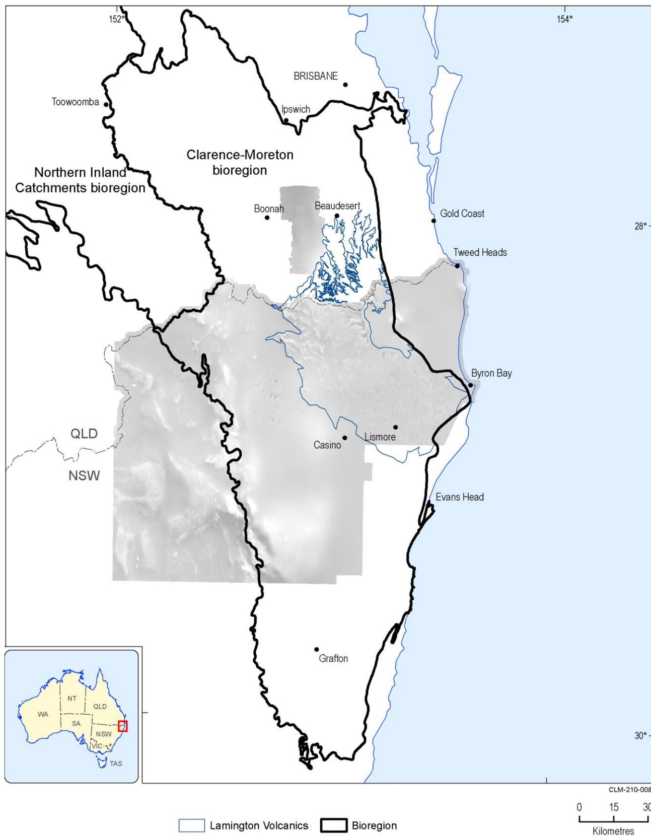
**Figure 11 Airborne magnetic surveys in the Clarence-Moreton bioregion showing the extent of the Lamington Volcanics and structural features**
