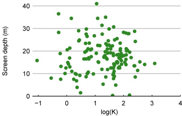
**Figure 51 Scatter plot showing the relationship between the screen depth and log(K) in alluvium, where K is hydraulic conductivity (m/day)**
