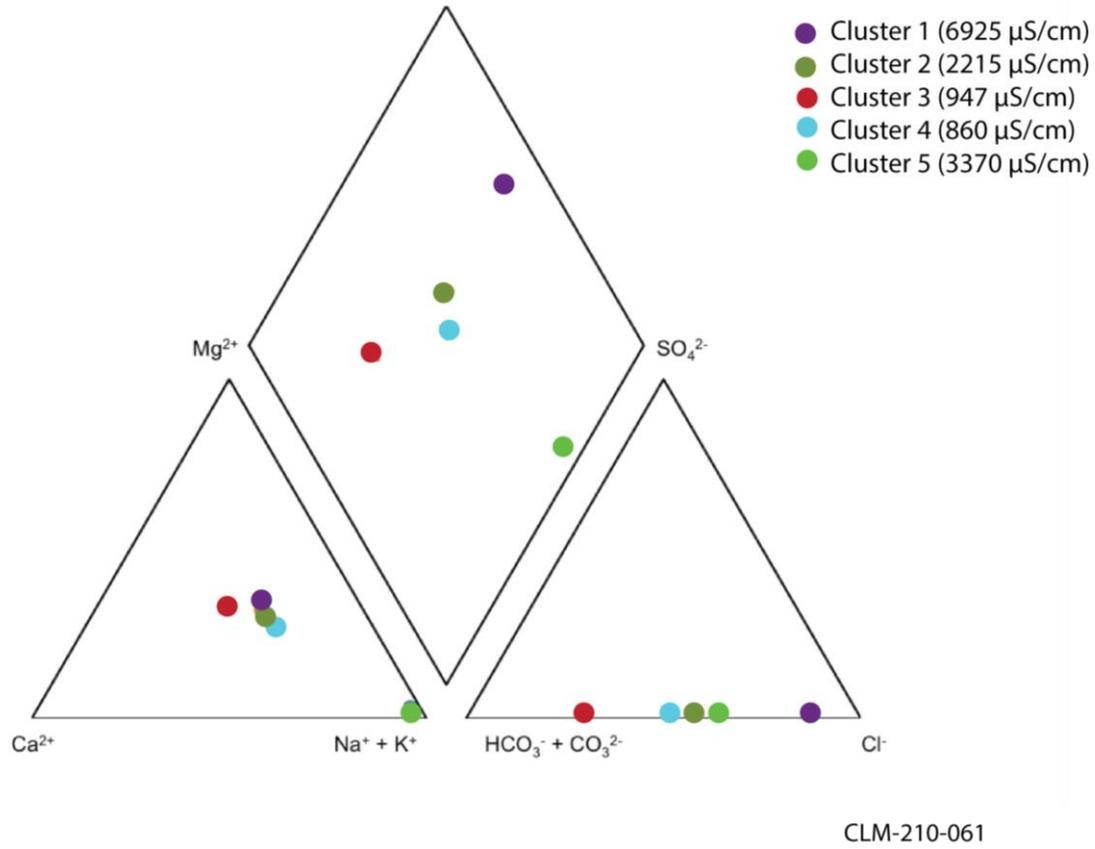
Figure 58 Piper diagram showing the major ion relationships of hydrochemical clusters in the Warrill creek catchment, Bremer and Logan-Albert river basins (based on median concentrations shown in Table 19)
