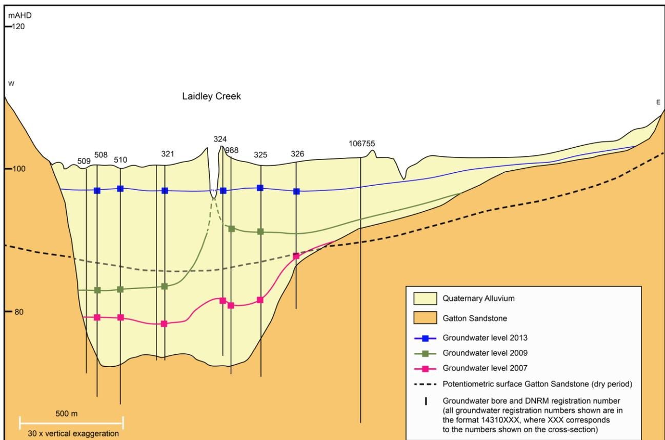
**Figure 66 Geological cross-section through the Laidley Creek catchment (subcatchment of Lockyer Valley)**
