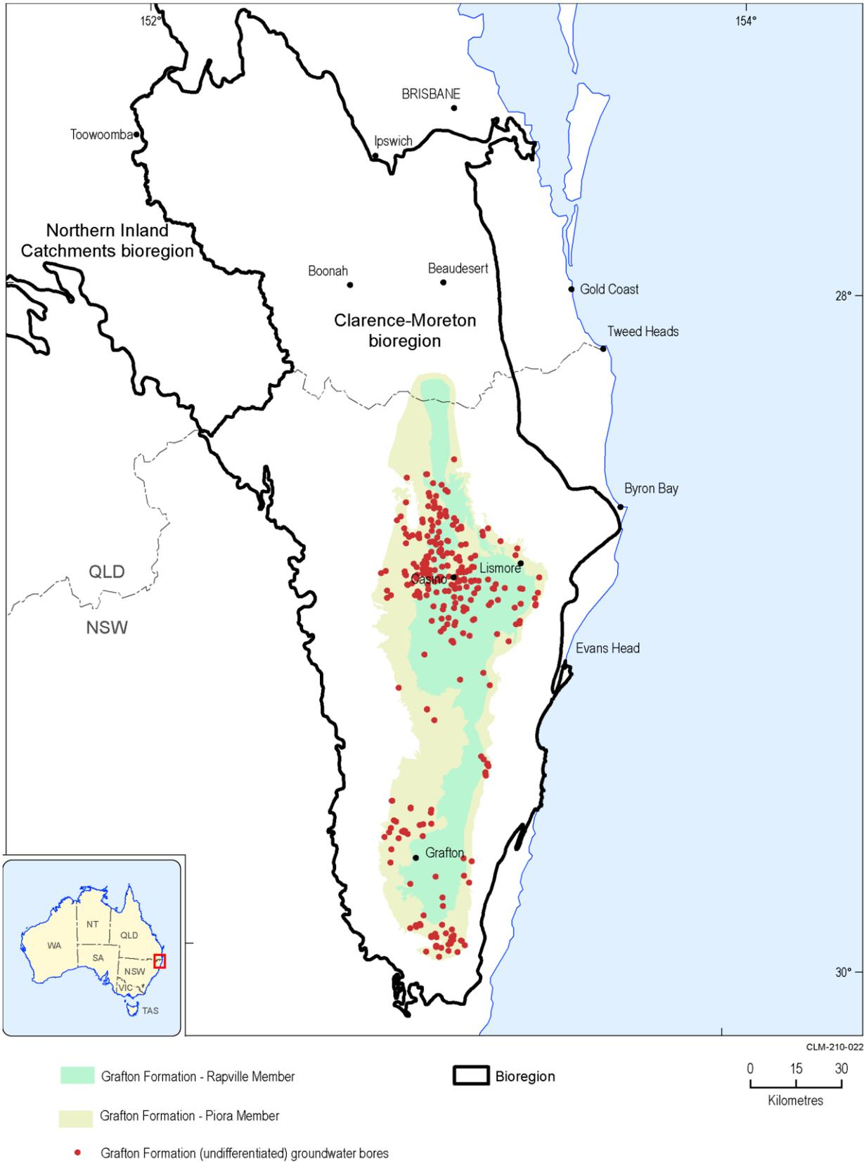
**Figure 24 Spatial distribution of bores with construction information in the Grafton Formation**
