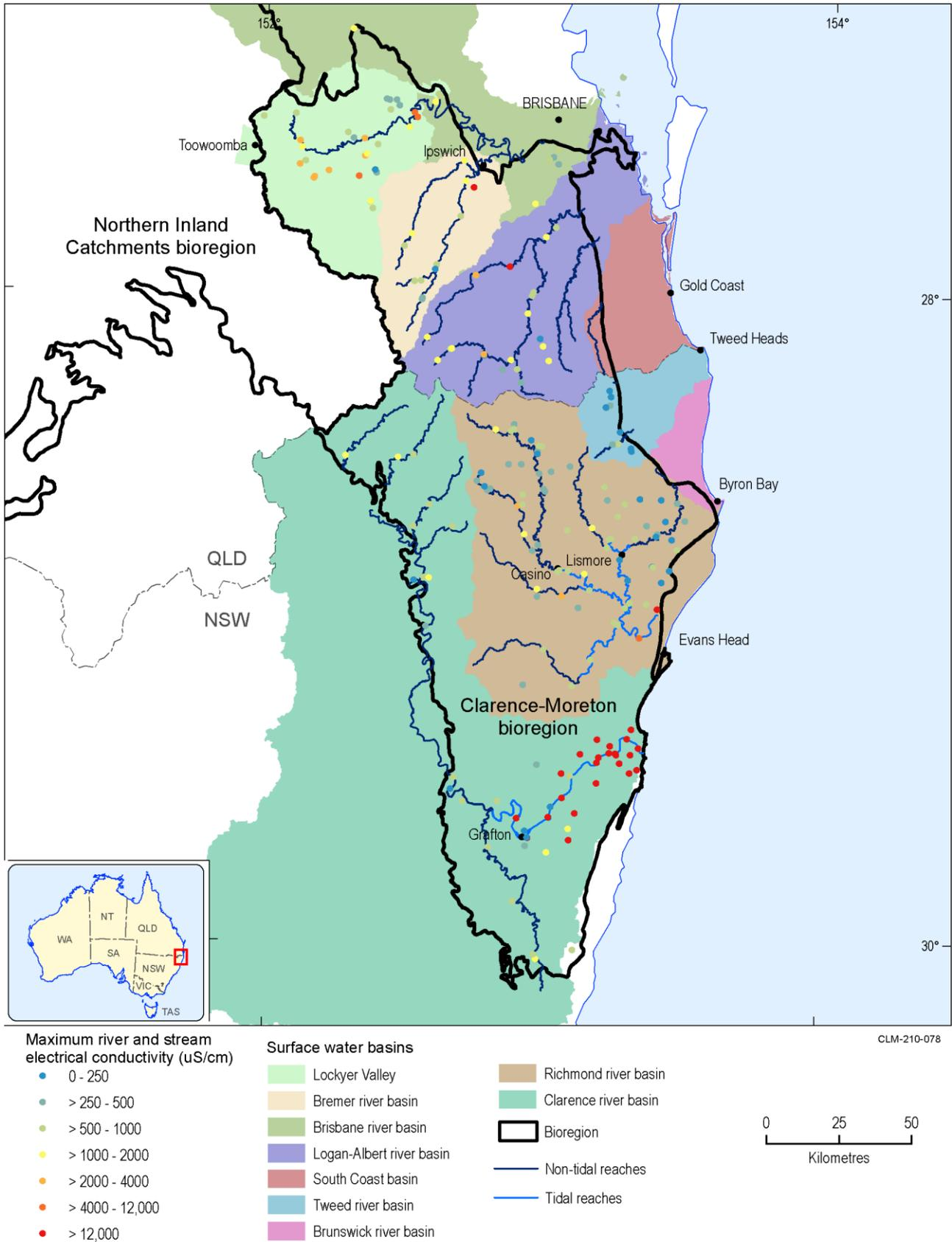
**Figure 64 Maximum stream electrical conductivity as representation of low streamflow conditions**
